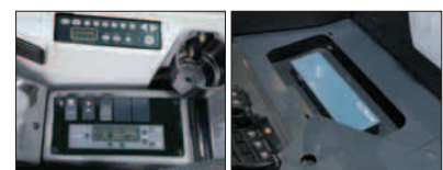
Air conditioner / AM-FM radio (Cab) Tool box (canopy)
